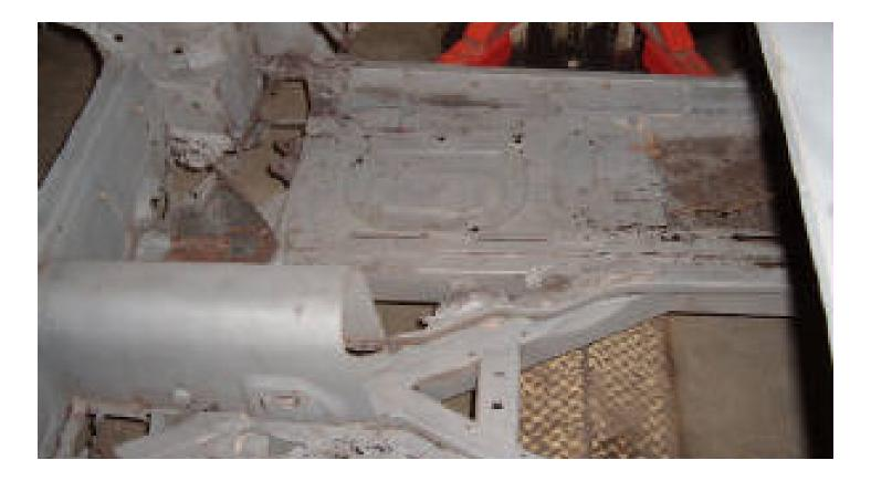
The completed chassis should be lightly blasted and immediately sprayed with primer, preferably zinc chromate based.
